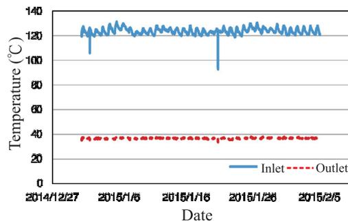
Fig.7. Air inlet and outlet temperature of AS3AC11S1 intercooler.
