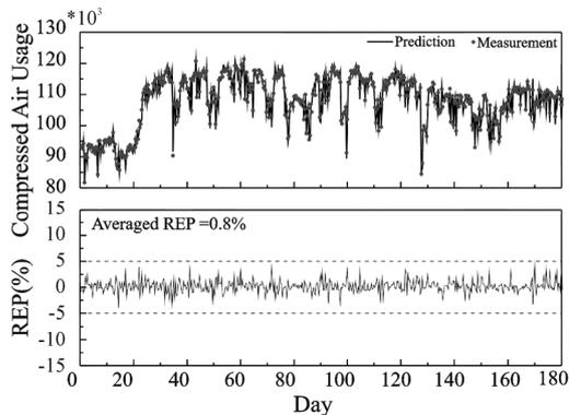
Fig.4. Prediction result of PA consumption after correction.
