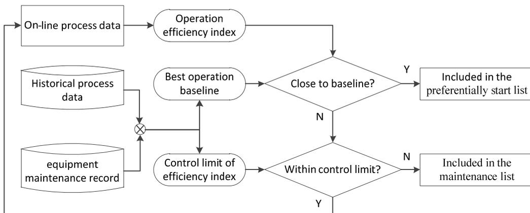
Fig.2. Flow chart of compressor and inter cooler monitoring.
