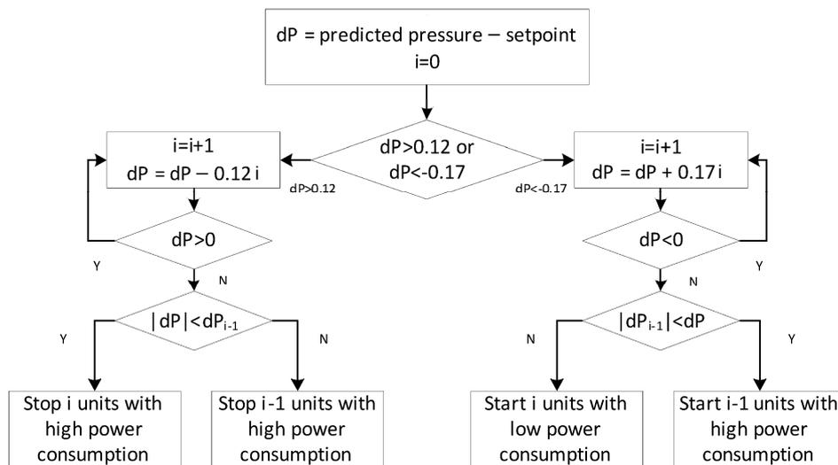
Fig.1. Algorithm of compressor loading and unloading.
