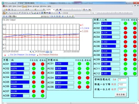
Fig.5. User interface of compressor optimal operation.
